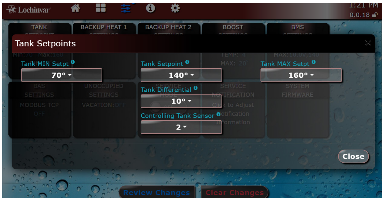
Figure 1-3 Tank Setpoints HW Screen
